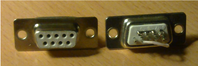
Figure 3. Simple loopback plug. For control signal loopback test connect pins (1, 4 and 6) and (7, 8 and 9) in two groups by three pins. For data test, connect pins 2 and 3.
